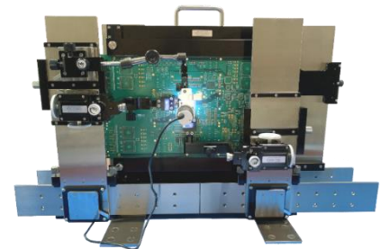
2-Sided Probe Station (VPS10)
